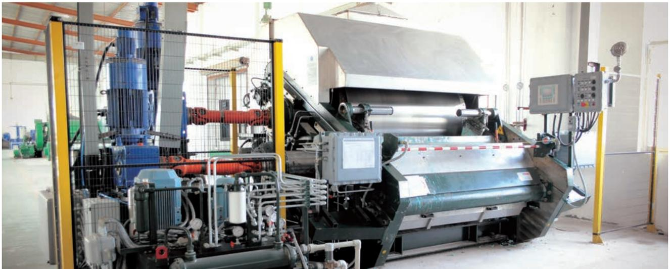
*Fully Automatic Compressed Fiber Sheet Manufacturing Line*
